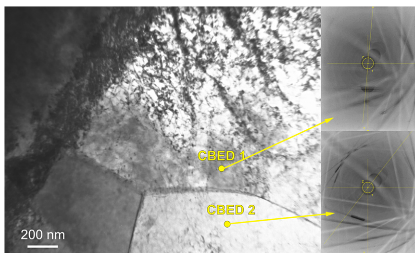
Fig. 8. Crystal lattices misorientation in neighboring dislocation cells of B2 austenite in sample C after ECAE (2 pass). CBED analyses in marked positions
